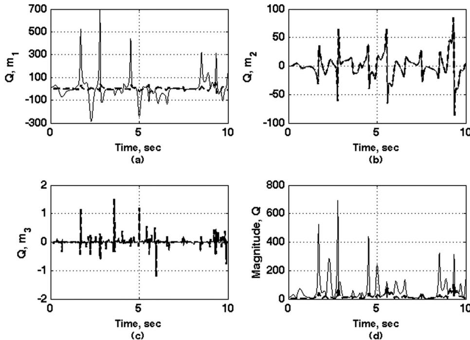
Fig. 11 Control forces (newtons) on the controlled actual system. The solid line shows the total control force,  $Q^T$ , and the dashed line shows the additional force,  $Q^u$ , needed to compensate for uncertainties in the actual system.
