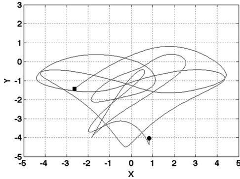
Fig. 9 Trajectory response (meter) of mass  $m_3$  over a period of 10 s of the controlled actual system when the uncertainties in the masses are prescribed as  $\delta m_1 = 0.1$  kg,  $\delta m_2 = -0.2$  kg, and  $\delta m_3 = 0.3$  kg and the uncertainty bound in Eq. (4.3) is chosen to be  $\Gamma(t) = 40$
