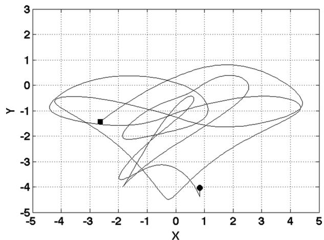
Fig. 2 Trajectory of mass  $m_3$  in the XY-plane (meter) of the triple pendulum shown for a duration of 10 s. The trajectory starts at the circle and ends at the square.
