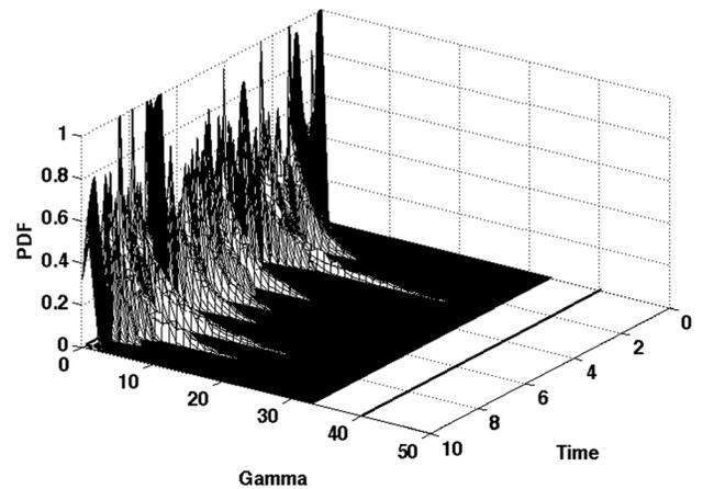
Fig. 8 Probability density function of  $\|\delta\dot{q}\|$  at each time  $t$  using Eq. (3.18) for the 1014 simulation points in which the masses have  $\pm 10\%$  uncertainties
