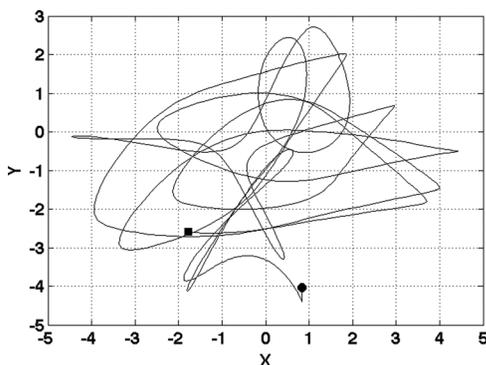
Fig. 5 Trajectory of mass  $m_3$  of the actual system over a period of 10s. The masses are  $m_1 = 1.1$  kg ( $\delta m_1 = 0.1$ ),  $m_2 = 1.8$  kg ( $\delta m_2 = -0.2$ ), and  $m_3 = 3.3$  kg ( $\delta m_3 = 0.3$ ). The system satisfies the energy constraint in Eq. (2.15).
