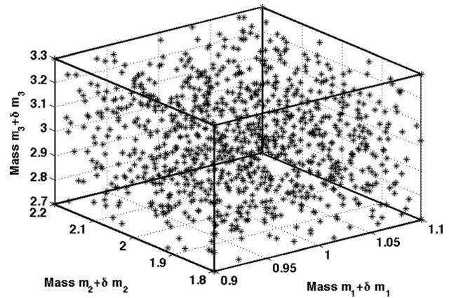
Fig. 7 The three masses  $m_i \pm \delta m_i, i = 1, 2, 3$ , of the actual system lie somewhere in the box shown. The figure shows 1014 uniformly distributed random points generated from a Monte Carlo simulation.
