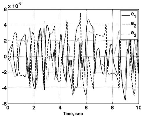
Fig. 10 Tracking errors between the controlled nominal system and the controlled actual system ( $e_i(t) := \theta_i(t) - \theta_{c_i}(t)$ ,  $i = 1, 2, 3$ ) in radians of the masses  $m_1$ ,  $m_2$ , and  $m_3$
