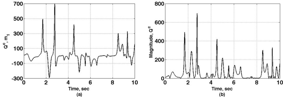
Fig. 4 (a) Control force applied to mass  $m_1$  of the nominal system to satisfy  $E = E_2 + E_3$ ; (b) magnitude of the control force. The control forces on masses  $m_2$  and  $m_3$  are zero.
