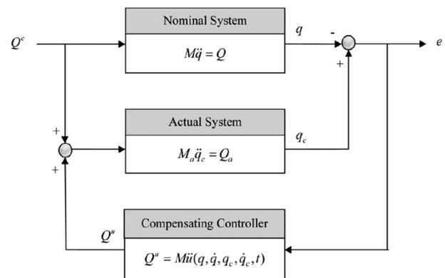
Fig. 6 The block diagram of the controlled actual system. Note that the compensating controller uses the mass matrix of the nominal system.
