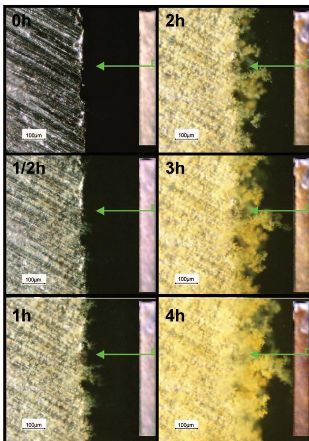
Figure 2. Time course comparison of rust detectability by light microscopy (left) and the unaided eye (right). The green square and arrow in the visible section denotes the area that corresponds to the microscopic image.
