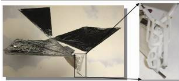
Fig. 17 Assembled MAV containing in-mold fabricated mechanism
