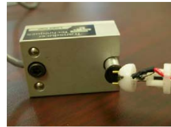
Figure 10. End-Effector Force Measurement using a GSO-10 Load Cell
